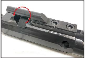
10. Remove the cam pin by lifting it out and away from the bolt and bolt carrier.
