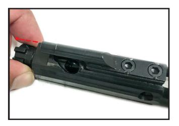
12. Depress the buffer, maintaining pressure as the buffer is under spring tension, to prevent it from being ejected when the buffer retainer pin is depressed.
