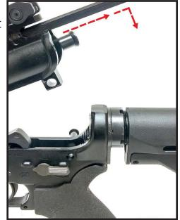
**7**. Push in the firing pin retaining pin from right to left of the bolt carrier group and remove the pin by pulling it out to the left.
