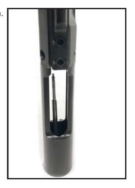
9. Push the bolt in towards the carrier until bolt rotattes and comes to a stop, then turn the bolt cam pin through 90 (i.e., at right angles to its normal position.
