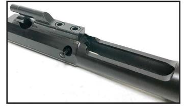
8. Tilt the bolt face up and remove the firing pin.
