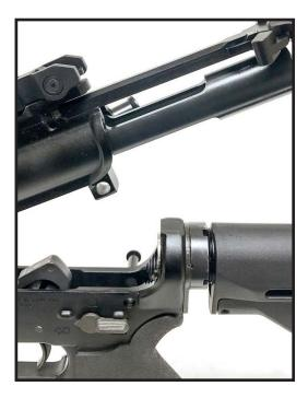
6. Remove the charging handle by pulling it backwards the keyway and then down and out of the upper receiver.
