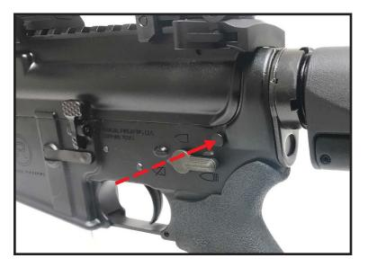
3. Pivot the lower receiver down and away from the upper receiver.
