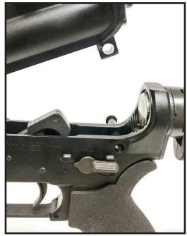
4. If required for more convenience, completely separate the upper receiver from the lower receiver by pressing the front take down pin from the left hand side of the lower receiver and pulling out the pin on the right hand side of the receiver until it comes to a positive stop.
