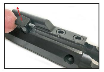
11. Pull the bolt forward and remove it from the bolt carrier.
